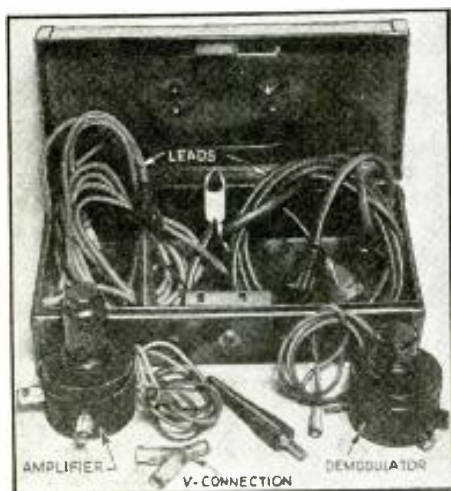
Fig. E. The accessories Mr. Maggio uses include Amplifier and Demodulator units shown by diagram in Fig. 1 (upper-right), pg. 343, December 1938 Radio-Craft, at B and A, respectively.
