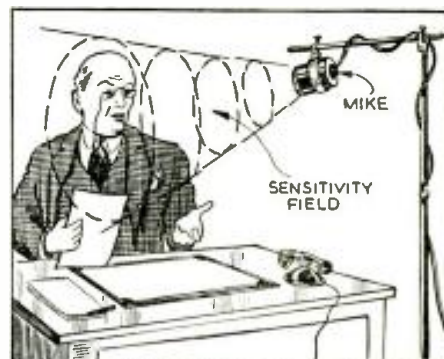
Fig. 3. How to keep the mike out of the camera field and yet within easy earshot of the subject's voice.
