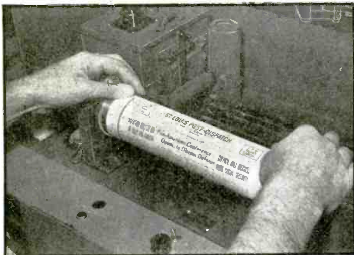
3 Here you see the master copy being placed on the scanner drum for transmission. The drum turns at the rate of 75 turns per minute. The present experimental transmissions have a fidelity of 125 lines per inch. A photocell is the light-variation pick-up unit.
